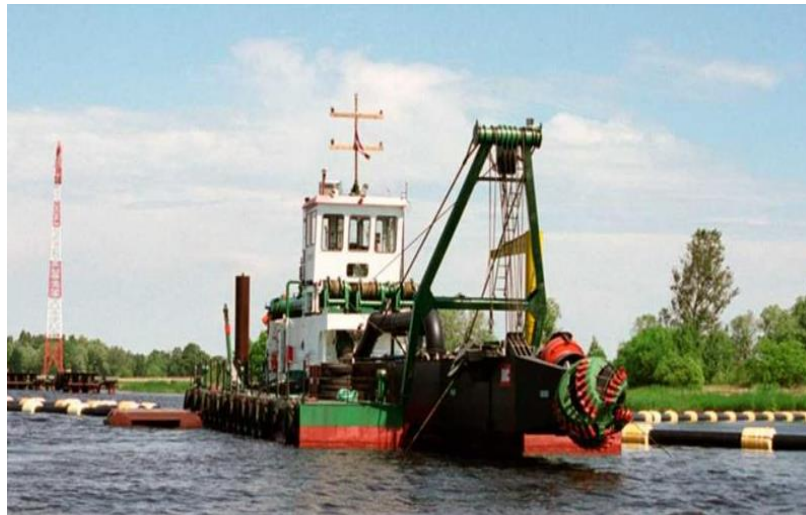
Gambar 2.6 Cutter Suction Dredge (CSD) (Sumber: Lutfie, 2017)
