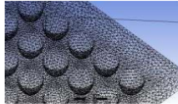
Figure 4. Detail of Meshing of the dimpled plate
