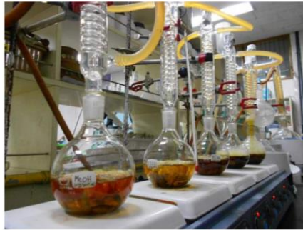
Gambar 4. Metode Refluks (Nugroho, 2017)
