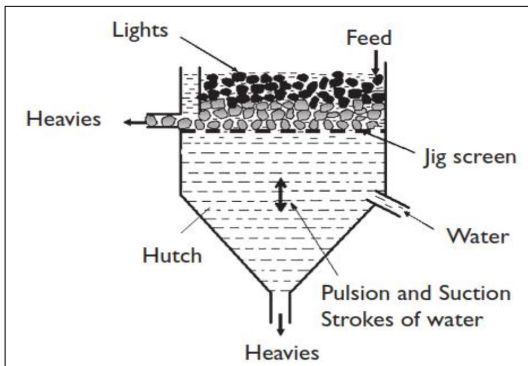
**Figure 2.2** Basic construction of a Hydraulic jig (Rao & Gouricharan, 2016).
