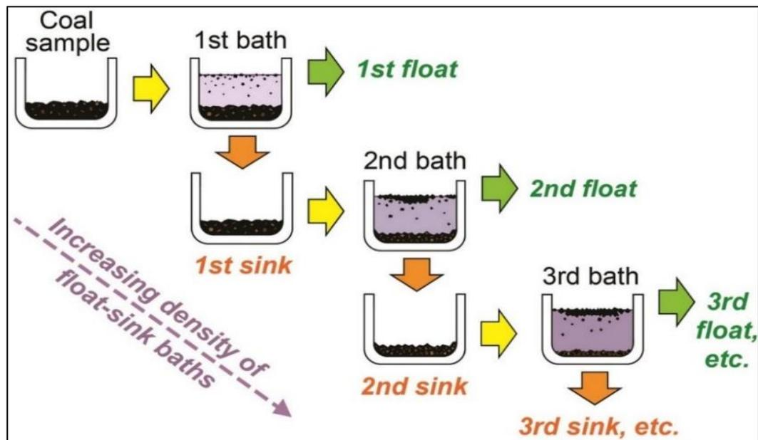
**Figure 2.4** Illustration of coal sink-float test (Survey, 2020).
