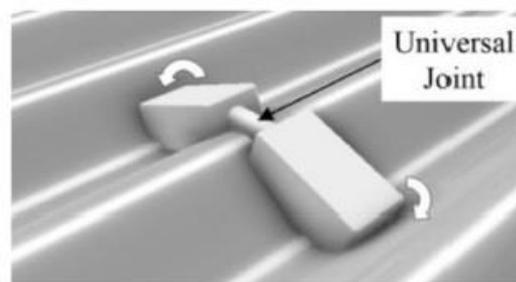
Gambar 3. Konsep wave activated body (Mustapa, M.A. et al., 2017)
