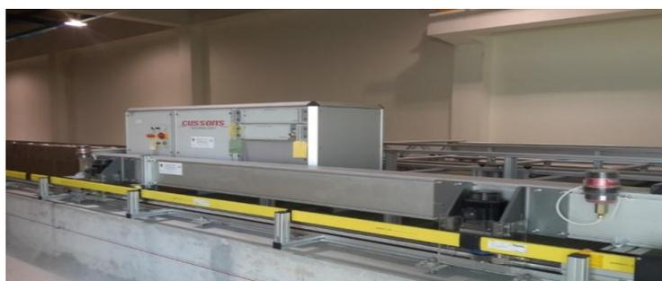
Gambar 16. Alat Penarik Model ( *carriage* )
