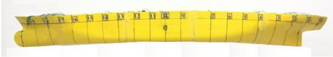
Gambar 26. Model *hydroelastic body*
