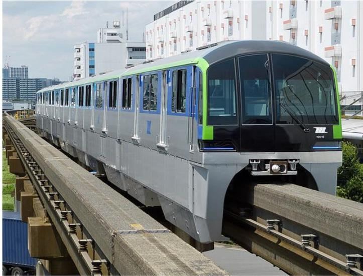
*Gambar 2.3 Tipe Straddle-Beam, Tokyo Monorail 10000 series EMU.*
