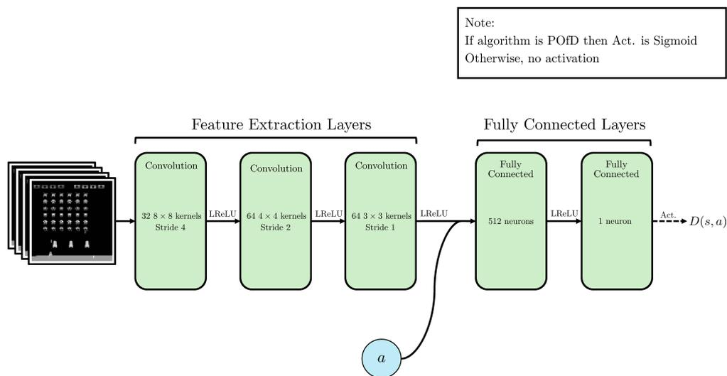
**Figure 3.4:** A visualization of the implemented discriminator network.
