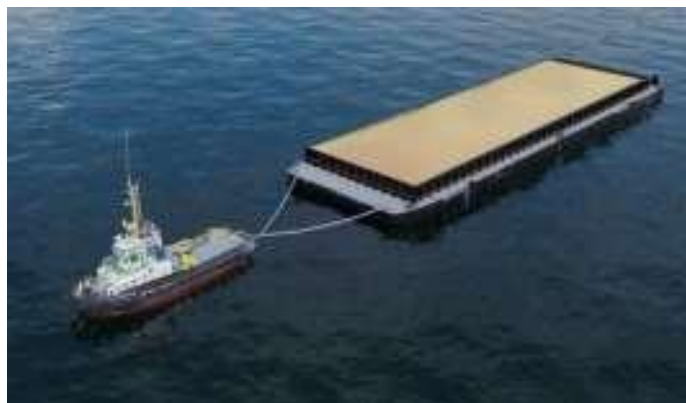
Gambar 2.6 Dry Bulk Cargo Barge [5]
