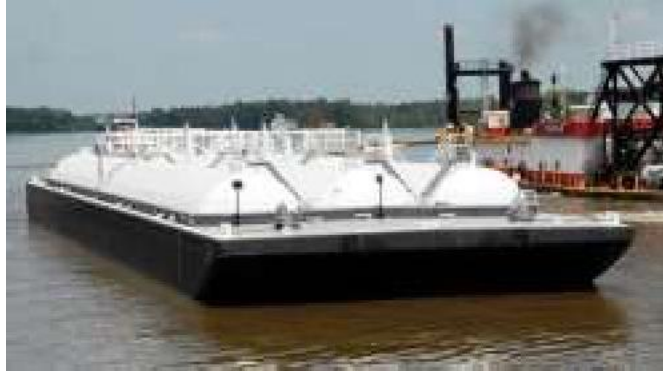
Gambar 2.7 Liquid Cargo Barge [5]
