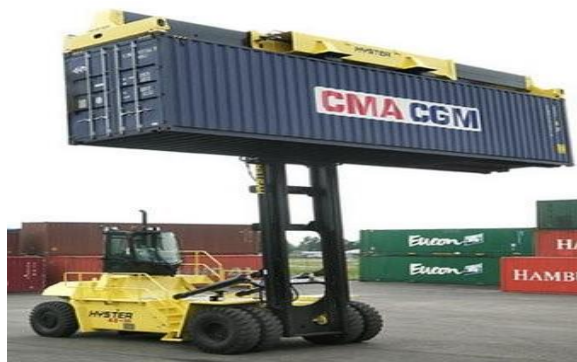
Gambar 18. Container Forklift (Sumber: airportassistant.wordpress.com )
