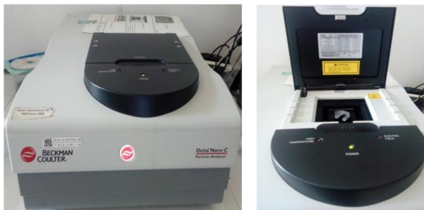
Foto 4. Instrumen particle size analyzer Beckman Coulter Delta Nano C Particle Analyzer
