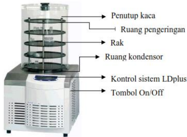
Gambar 3. Freeze dryer Christ alpha 1-4 LD-plus (Sumber: Mortazavian dkk, 2007).
