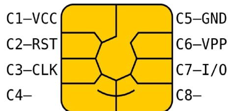
Gambar 9 Smart Card's pin contact
