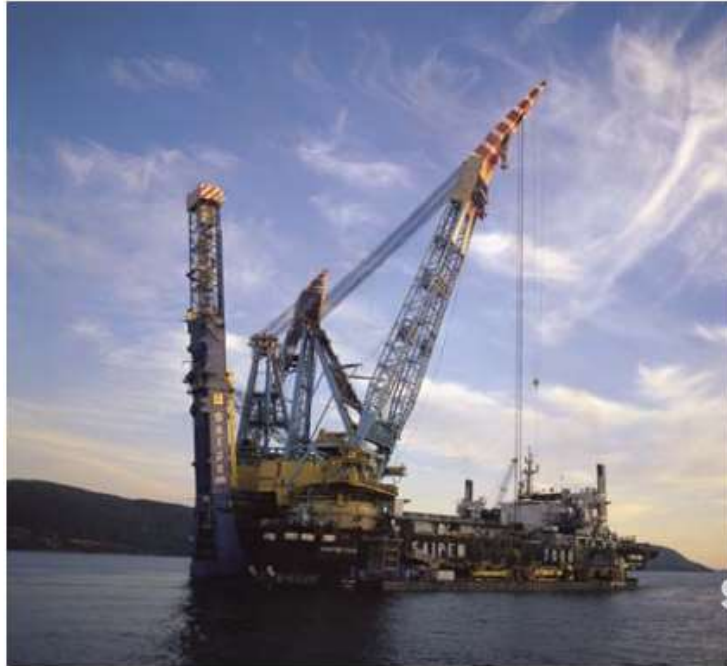
Gambar 2 Saipem S7000 (SSCV with maximum of 1400 ton Capacity).
