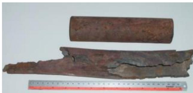
**Gambar 2. 24** *Tube Superheater Boiler* kelapa sawit
