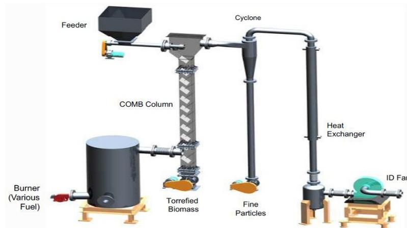
**Gambar 2. 10** Bagian-bagian reaktor Counter Flow Multi Baffle (COMB).
