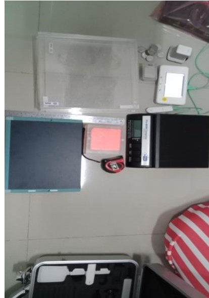
Lampiran 1. Multimeter X-Ray, Derektor, Pantom, Meteran, koin, filter Al.
