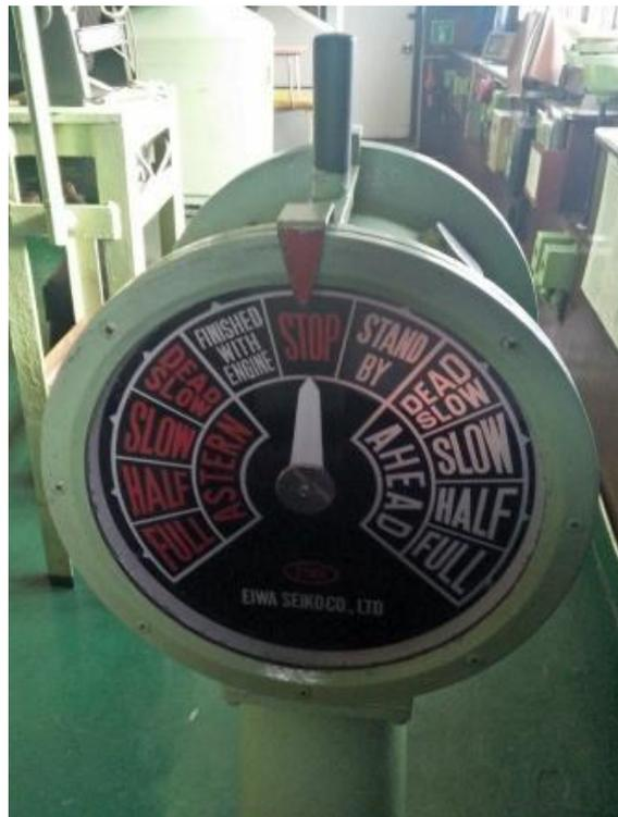
Gambar 2.13. Engine Telegraph
