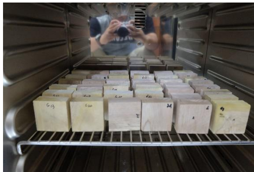
Gambar 5. Proses pengujian Kadar Air
