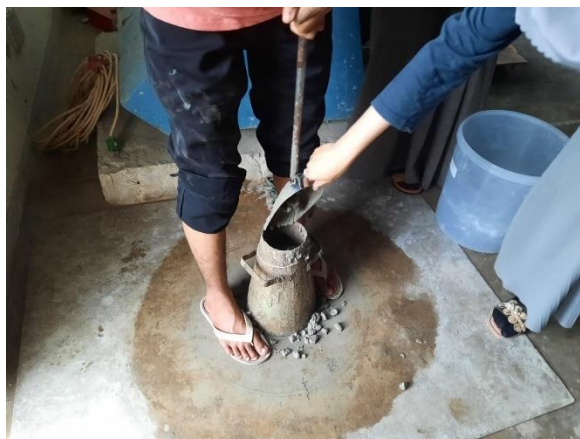
Pengujian nilai slump beton normal
