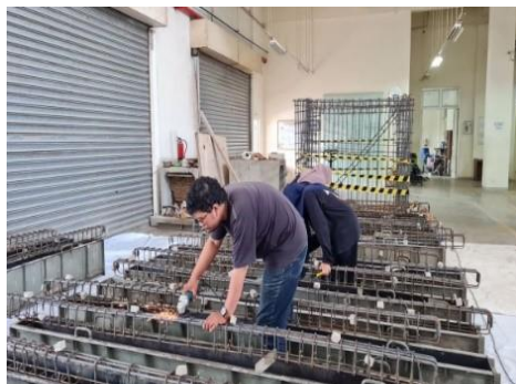
(c) Pemasangan Strain Gauge
