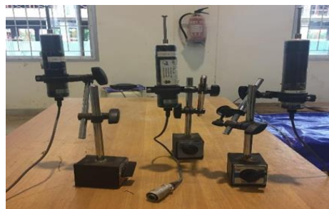
Gambar 21. LVDT ( Linear Variable Displacement Transducer )
