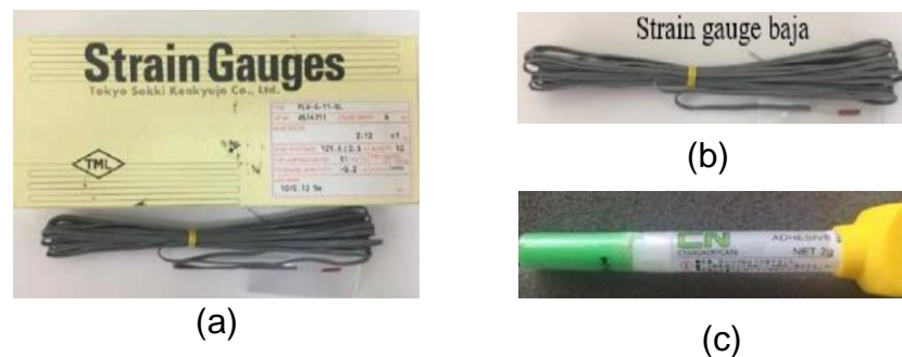
Gambar 18. (a) FLA-2-11 ( gauge factor 2,12\pm 1\% ), (b) strain gauge baja, (c) CN Adhesive
