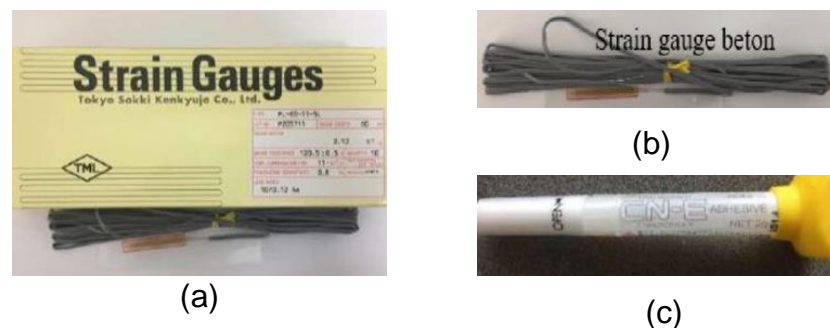
Gambar 19. (a) PL-60 11 ( gauge factor 2,09\pm 1\% ), (b) strain gauge beton, (c) CN Adhesive
