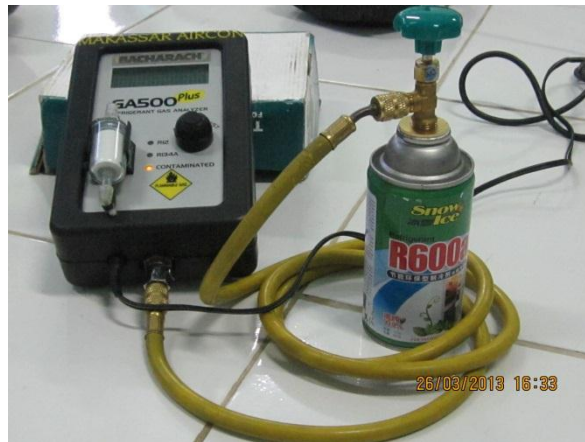
Gambar A.13 Refrigeran gas analyzer
