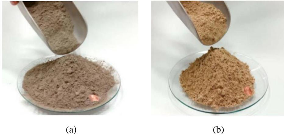
**Gambar 2. 3** (a). Fly Ash Kelas F; (b). Bottom Ash Kelas C
