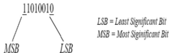
Gambar 2.2 Most Significant Bit dan Least Significant Bit
