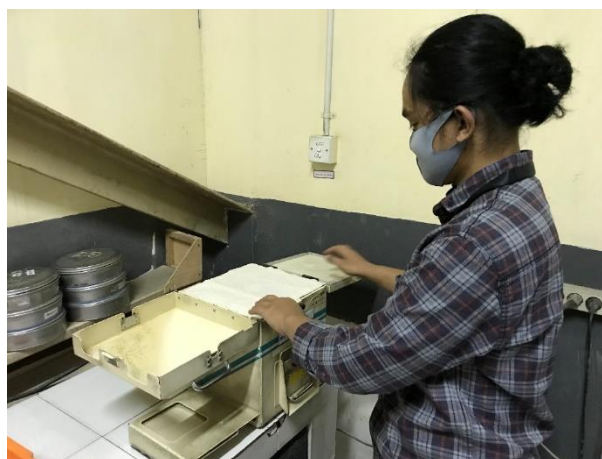
Keterangan: Uji Pellet Durability Index di PT. Japfa Comfeed Makassar
