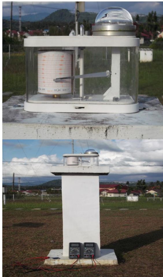
Gambar 3.2 Alat Ukur Radiasi Matahari Actinograph BMKG Kaiwatu Manado
