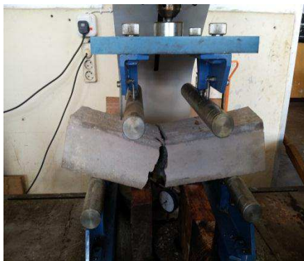
(a) Beton nonfiber
