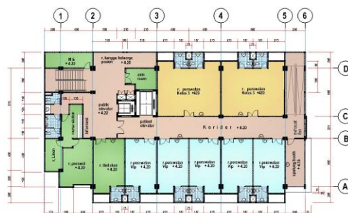
Gambar 2. 9 Denah Typical Lantai 3,4,5
