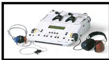
Gambar 12. Alat-alat Audiometer (Lassman et al., 2014).
