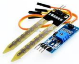
Gambar 2-2. Sensor Higrometer Soil Moisture YL-69
