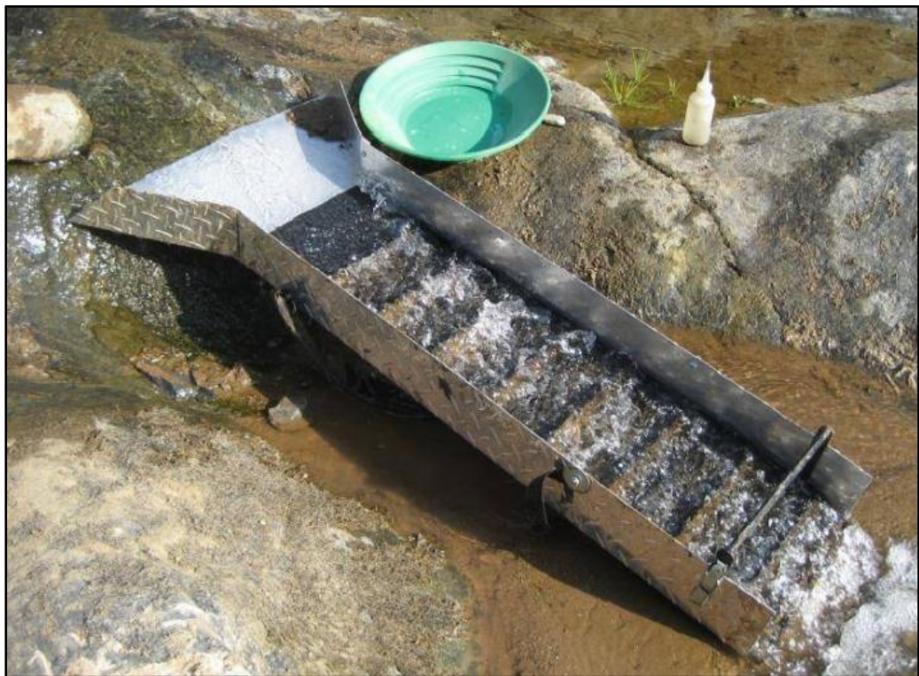
Gambar 2.7 Sluice box aluminium (Ludiansyah, et al. , 2018)
