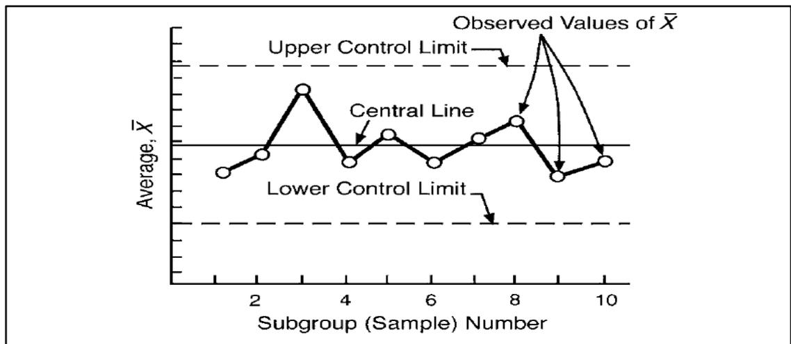
Figure 2.3 Control chart (ASTM International, 2010)
