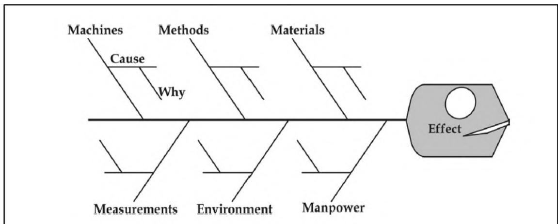
Figure 2.4 Cause and Effect diagram (Kiran, 2017)
