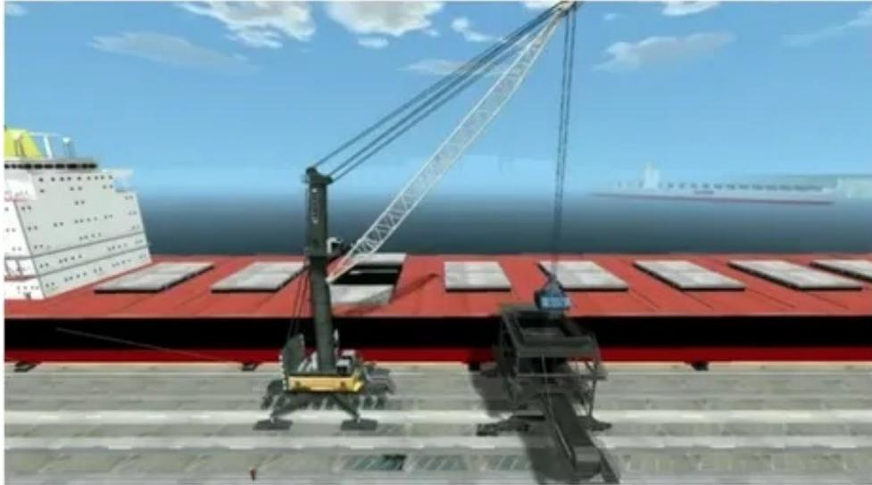
Gambar 2.12 *Harbor mobile crane (HMC)*
