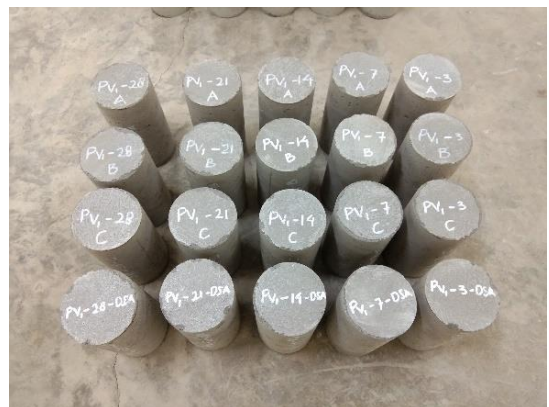
Benda Uji Paving Block PV 1 30% Limbah Gypsum Board
