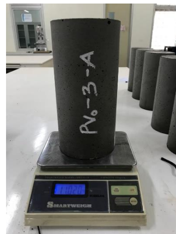
Penimbangan Berat Benda Uji Paving Block PV 1 30% Limbah Gypsum Board
