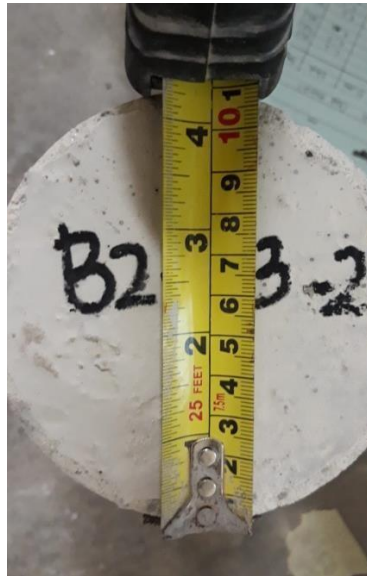
Mengukur diameter beton
