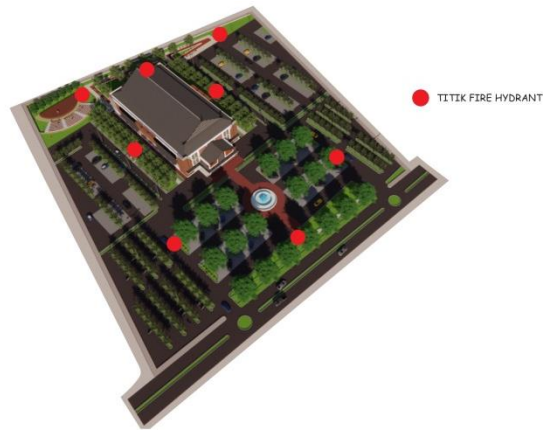
Gambar 7 Titik Fire Hydrant
