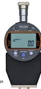
GSD-719K-R Type A Durometer Digital type Stand mounting compatible type Peak pointer type
