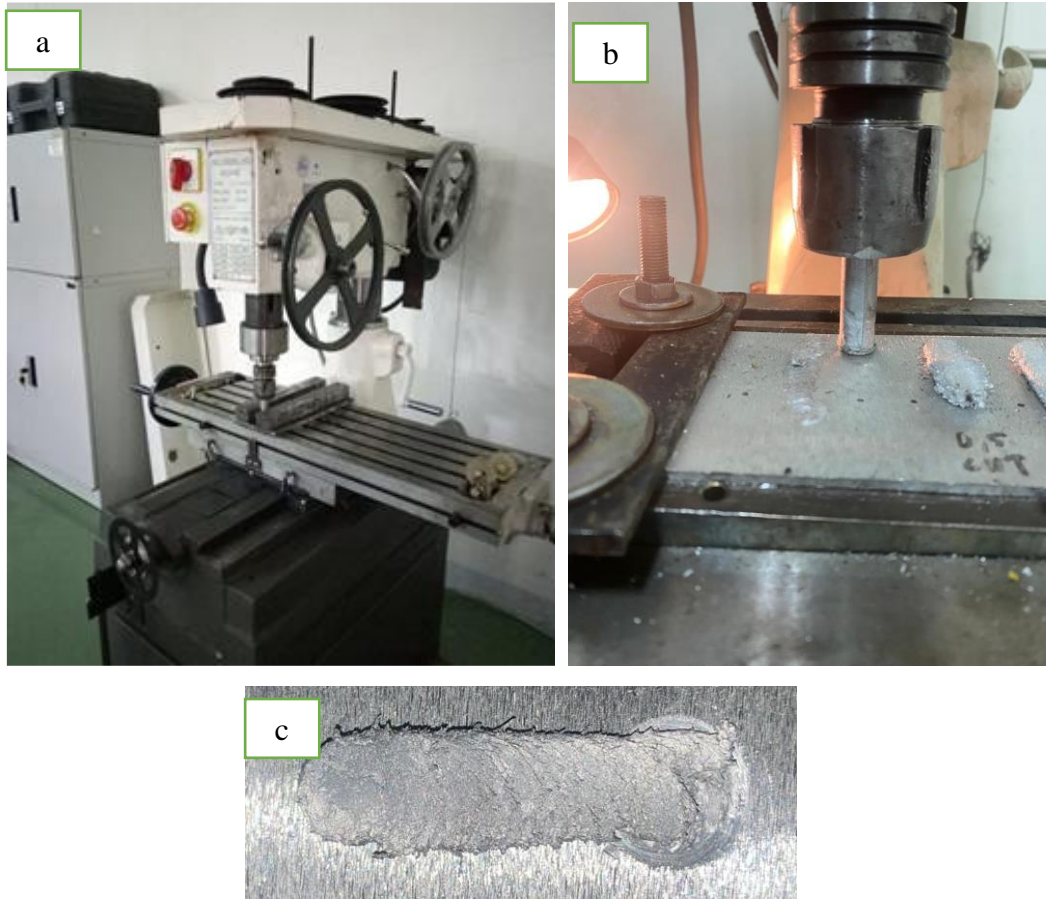
Gambar A.8 Proses friction surfacing (a) mesin Drilling-Milling Lc-40 A (b) proses friction surfacing (c) Hasil friction surfacing
