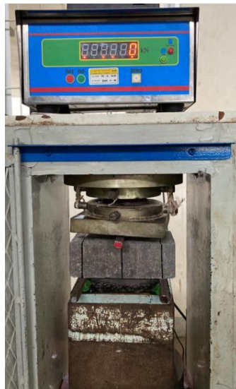
Gambar 4. Pengujian Kuat Lentur Paving block
