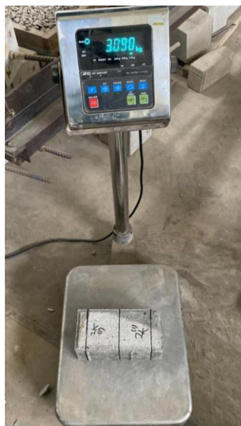
Gambar 5. Pengujian Berat volume Paving block
