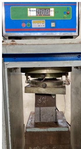
Gambar 3. Penhujian Kuat Tekan Paving block
