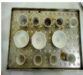
Lampiran D.5 Pengujian Kadar Abu
