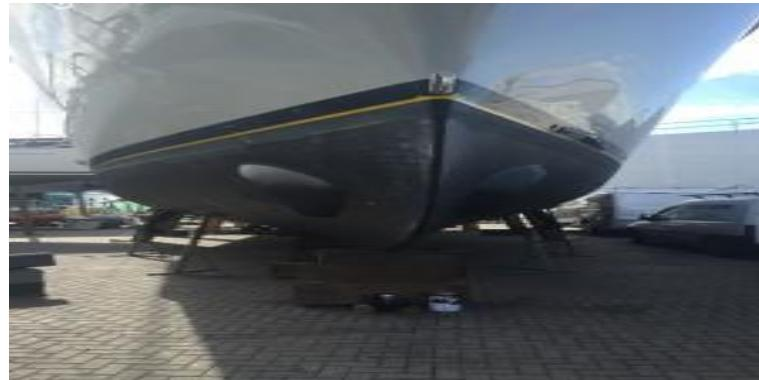
Gambar 2.5. Displacement Ship
