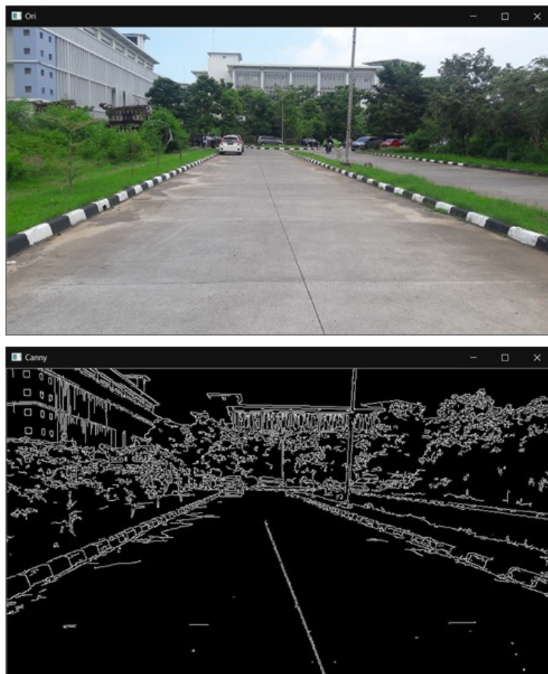
Gambar 9. Deteksi Tepi ( Canny ) T1 = 100 , T2 = 250 .
