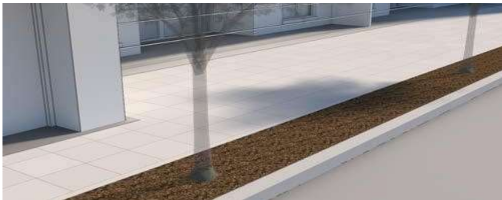
Gambar 18. Parit Terbuka ( Open Soil Trench ) (Sumber : Complete Streets Design Guide, 2017)
