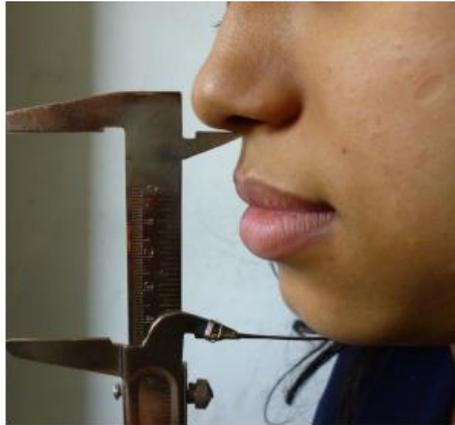
Gambar 2.1: Pengukuran dimensi vertikal menggunakan jangka sorong yang dimodifikasi (sumber: Basnet B, Parajuli P, Singh R, dkk. *An anthropometric study to evaluate the correlation between the occlusal vertical dimension and length of the thumb Clinical, Cosmetic and Investigational Dentistry* 2015:7.)
