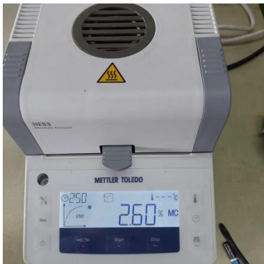
Gambar 14. Evaluasi kandungan lembab granul. Alat Moisture analyzer (Merek Mettler Toledo HE73).
