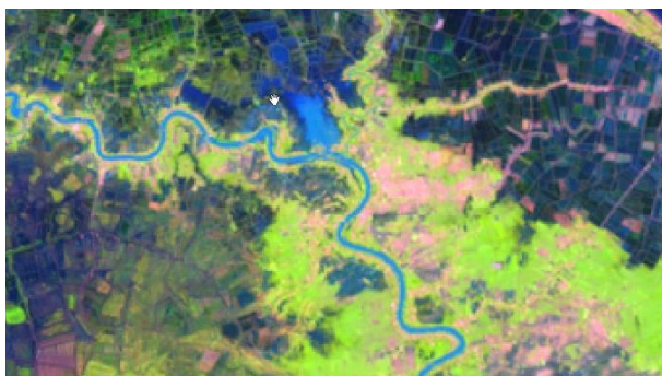
Composite Band 5,4,3 on Landsat 7 in green to identify agriculture
