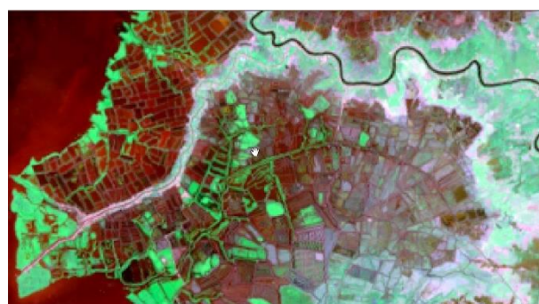
Composite Band 4,5,6 on Landsat 8 with green highlighter to identify mangroves
