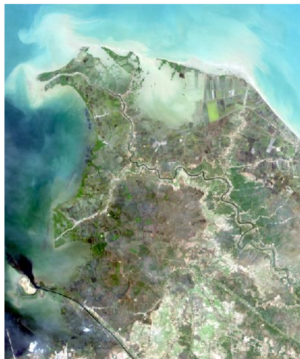
True Color can use Composite Band 4,3,2 on Landsat 8
