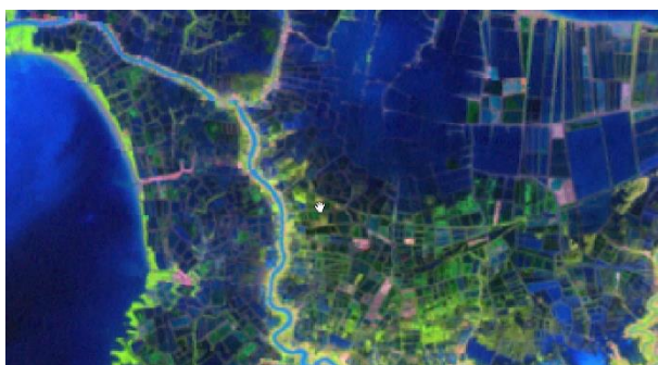
Composite Band 5,4,3 on Landsat 7 with blackish blue color to identify ponds
