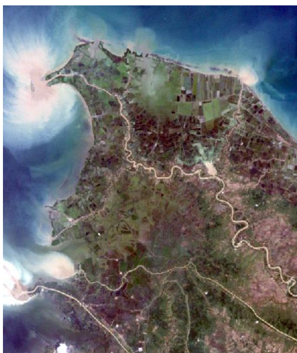
True Color can use Composite Band 3,2,1 on Landsat 7
