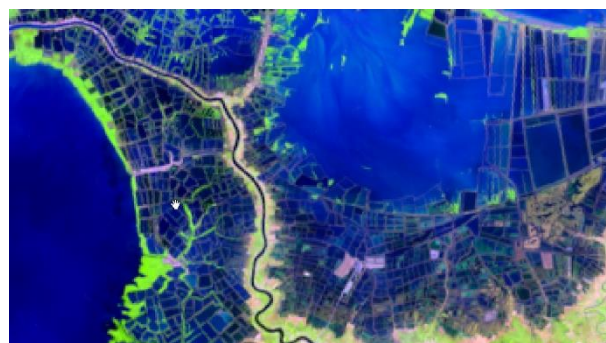
Composite Band 6,5,2 on Landsat 8 with blackish blue color to identify ponds
