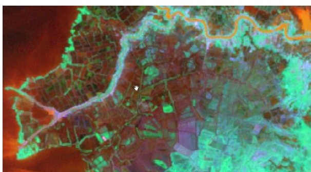
Composite Band 3,4,5 on Landsat 8 with green highlighter to identify mangroves
