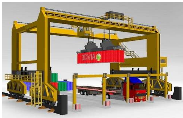
Gambar 2.3 Rail Mounted Gantry Crane (RMGC)
