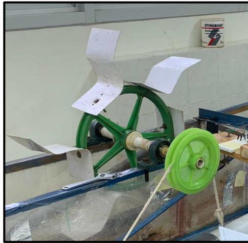
Gambar C1. Turbin Air Sudu Bengkok 45° Material Sudu Plastik
