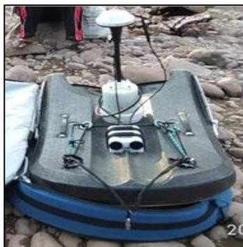
**Gambar 6.** *Acoustic Doppler Current Profiler ( ADCP)*
